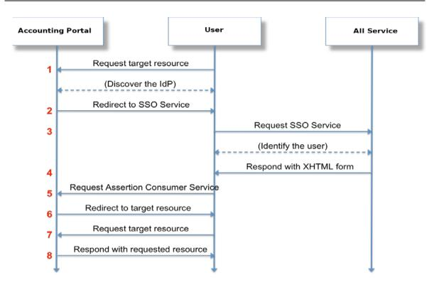
Figure 7: SAML Authentication Mechanism
